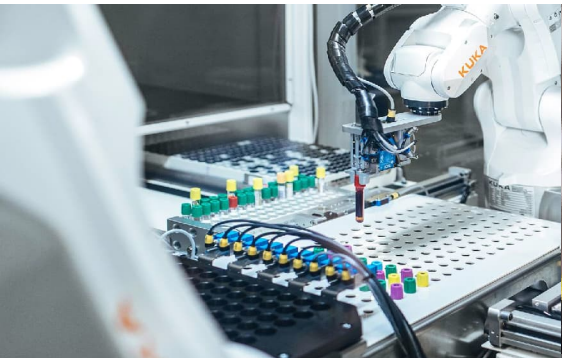
Robot arm for sorting of blood samples by hospital personnel and e
