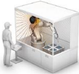
Intrusion detection with vertical installation
